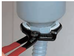
With square jaws fitted, grips large plastic nuts securely.
